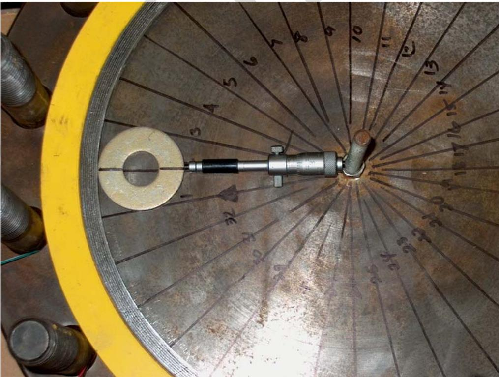
**Figure 3. Radial Measurement of Gasket Inside Dimension
